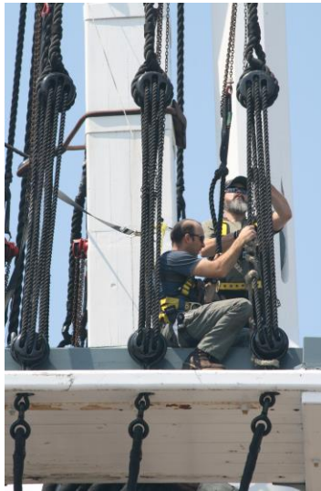
Riggers Ryan Whitehead and Steven Ridlon set starboard fore topmast lanyards, July 2017
