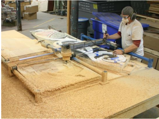
Joshua Ratty using GEMINI Universal Carving Duplicator replicating Constitution's 1930 trailboards, April 2017 14
