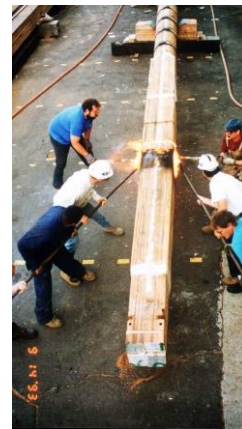
New lower fore, main, and mizzen masts were made by the Detachment
